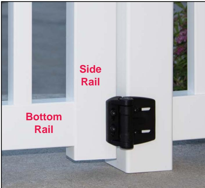
**Gate Hardware:** If possible, it is best to install the gate hardware on the rails so the gate hardware screws are installed through the side rails and through the top/bottom rails. This provides a secure and stronger installation. It is best to drill pilot holes for gate hardware.
