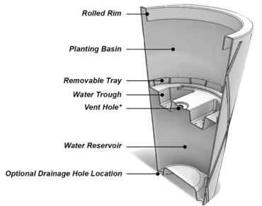
\* The vent hole in the center of the tray is part of the manufacturing process. It also serves as an internal drainage hole.
